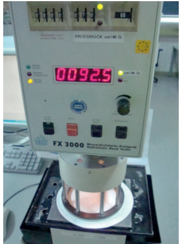
Picture 3: EN20811 (test equipment)
