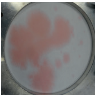
Grade 5: several leakages after 2 hrs (20 cm H 2 O) on max 50% of surface
