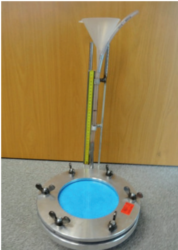
Picture 2: EN13859 W1 class (test equipment)
